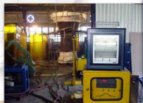
Recorder with heat cycle in progress
