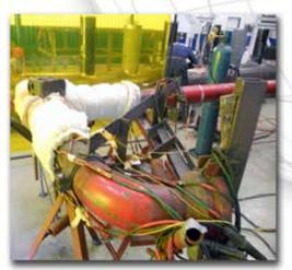
Allweld can pressurise test pieces to 2980 bar.
